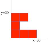
(note that if it is the y-axis you are moving from, the x-coordinate of the mass will tell you how far you are from the y-axis). Do this for all the masses in the system, add those weighted position ("mx" quantities) and divide by the total mass in the system. Do that for both axes and you will have the twodimensional coordinate for the system's center of mass.
